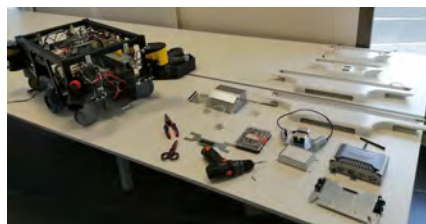
(h) Final figure depicting the main components contained inside of the MiR100 robot, alongside the tools used for the teardown.
