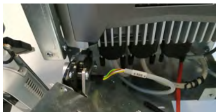
(g) The on-board controller is the embedded and "ruggedized" EC70A-SU from DFI which features an Intel processor and a Ubuntu 16.04 file system.
