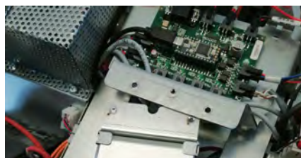
(e) Under an RF cage we find a Teensy board for LED control and a third party speaker to play the sounds from the on-board controller.
