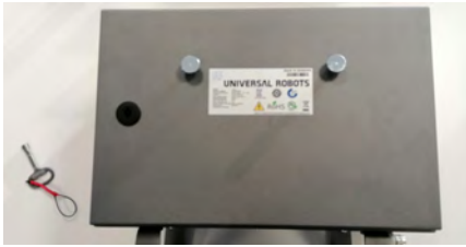
(a) Universal Robots URe3 controller. The controller has a mechanical lock aimed to prevent ingress to the internals from non authorized parties.
