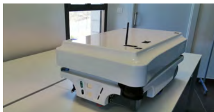
(a) The top shell sits on top of a metal frame that protects all the electronic components. Simply lifting the top shell reveals the internal electronic components.
