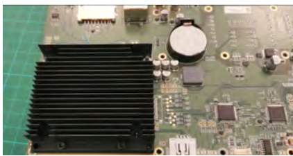
(h) Under the heatsink we find a MSC Q7-BT module on an ECX form factor and an Intel SoC with DDR3L memory.
