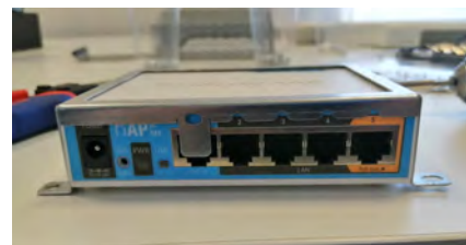
(i) Both the safety programmable logic controller (PLC) and the on-board controller are connected to a Mikrotik hAP ac. A 2.4/5GHz dual-band omnidirectional access point.
