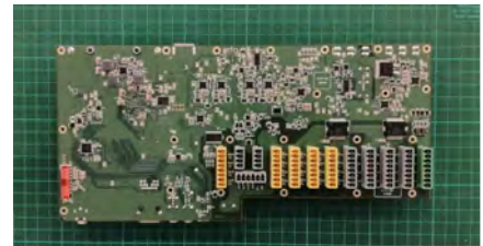
(f) Unlike previous hardware iterations, the e-Series controller presents both the safety logic and the control logic merged into a single PCB. See Figure 5 for a simplified diagram.
