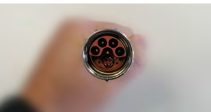
(k) Even though the pin-out is quite similar to previous iterations of the CB3 controller, the connector itself has a different shape
