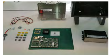
(i) Final figure depicting all the components contained inside of the Universal Robots URe3 controller, leaving aside the teach pendant.
