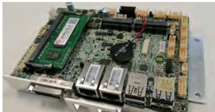
(d) No secondary memory is located on the printed circuit board (PCB) besides minor non-volatile memories and the USB stick we found connected outside.
