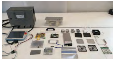
(i) Final figure depicting all the components contained inside of the Universal Robots UR3 CB3.1 controller, leaving aside the teach pendant.
