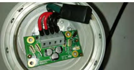
(j) Opening the base joint of the manipulator we find the connections coming from the controller the 48V leads and the micro-USB for data.
