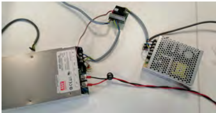
(h) A safety relay and two power supply units (PSUs) identified, one for the compute logic (12V) and another one to power the actuators (48V).
