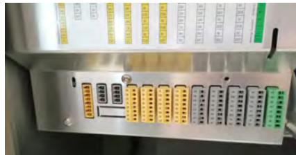
(e) The safety side of the controller (documented in the user manuals) includes quick connectors which can be removed by carefully wiggling them out.
