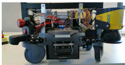
(d) The battery is enclosed in a steel box and held by a retaining plate to prevent movement and connected to a DP9 connector and DC 24V wires.
