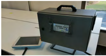
(a) Universal Robots UR3 robot CB3.1 controller and associated teach pendant (HMI). The controller has a mechanical lock aimed to secure physical access.
