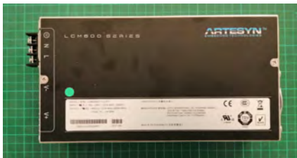
(e) The PSU is a Artesyn LCM600 series with an output of 48 V, and an input of 85–264 Vac. Has a typical full load efficiency of 89% up to 600 watts.
