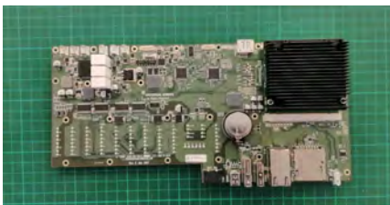
(g) DC to DC power management takes place on the board unlike previous iterations. The positions of the relays may hinder transistor cooling
