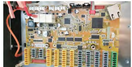
(f) After removing the metal shields, the safety board electronics are fully visible. The main logic is driven by an NXP LPC4437JET256 micro controller unit (MCU).
